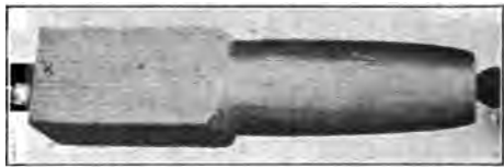
Fig. 249. First Step in Turning Footstool Leg.
